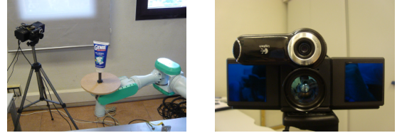
Figure 1. Left: PMD Camcube 2.0 coupled with a color camera. Right: Turn-table setup using a PA10 robot.
