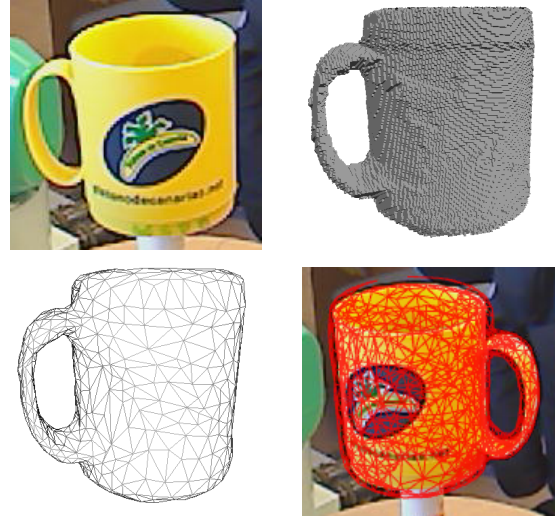
Figure 3. Example of acquired model: cup. Top left: object to scan, top right: carved volume, bottom left: Poisson reconstruction, bottom right: reprojection on a color image with known pose.
